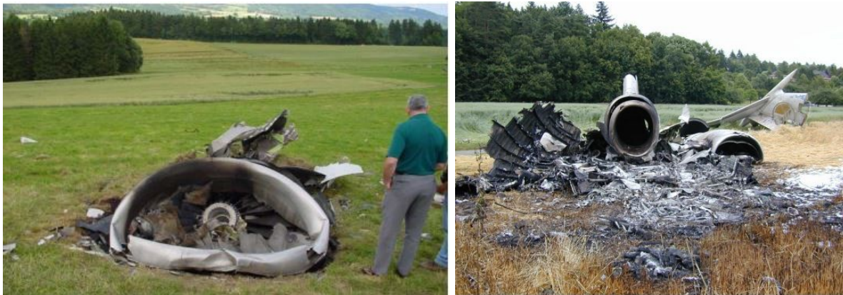
Figure 6 (Left): Wreckage on DHL Flight 611 (Boeing 757-23APF) Right Engine
