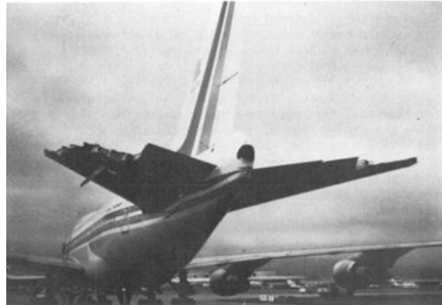
Figure 3: The damage caused by the upset during the 30,000 feet plunge.
