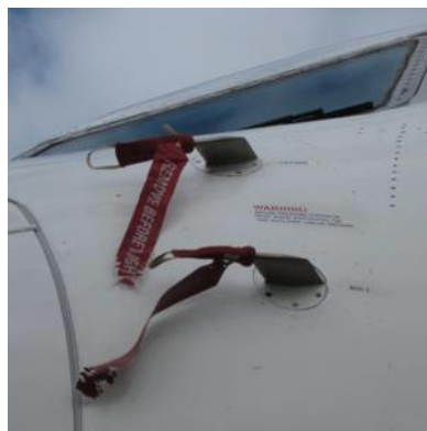
Figure 3: Pitot tubes on a B757, like the ones involved with the crash
